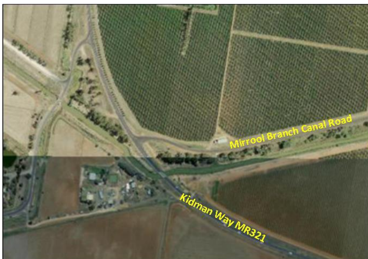
Image (above): Constraint 7.4 Griffith - Mirrool Branch Canal Rd intersection presents a sharp turn into fast traffic on a bend. Image from NSW LPI
