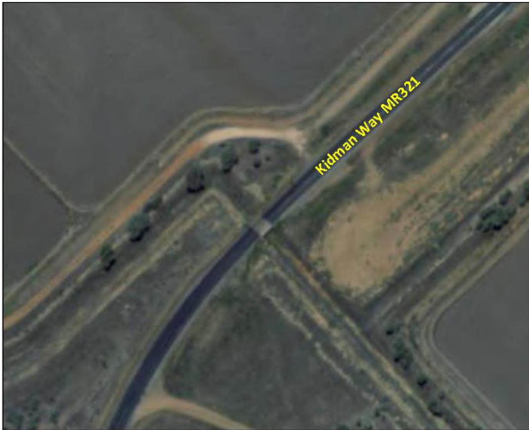
Image (above): Constraint 7.5 Griffith - Railway crossing has sharp approach and departure bends at Widgelli Silos
