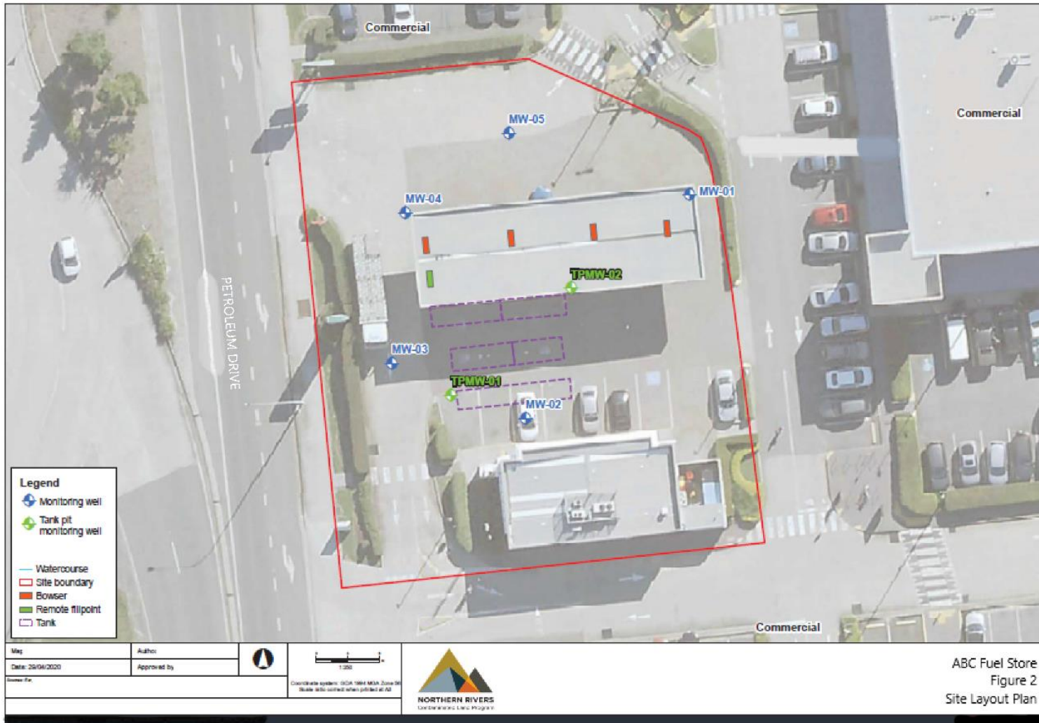
Figure 2 UPSS Site Layout Plan – Groundwater monitoring wells
