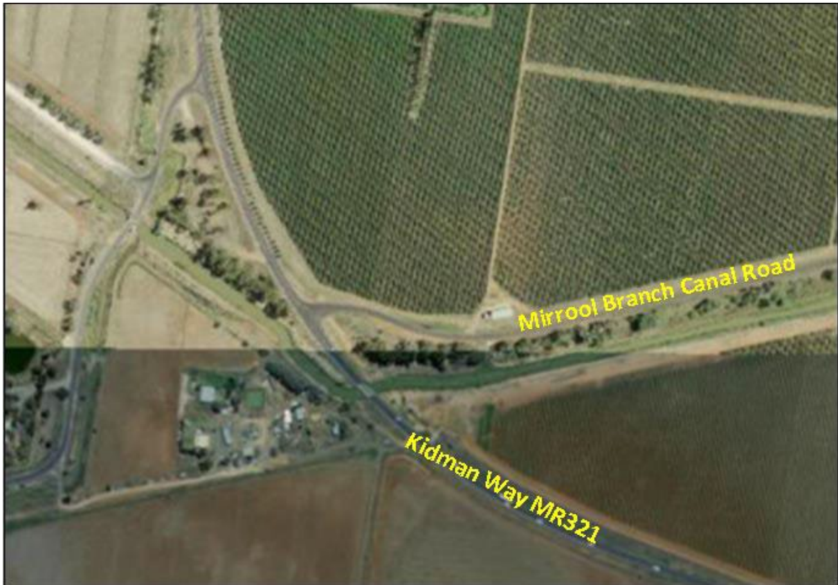
Image (above): Constraint 7.3 Griffith - Mirrool Branch Canal Rd intersection presents a sharp turn into fast traffic on a bend. Image from NSW LPI
