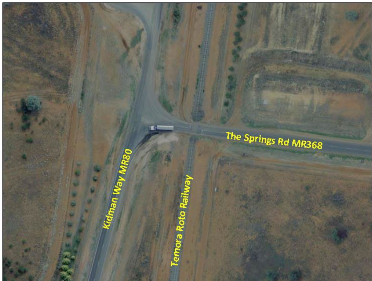
Image (above): Constraint 19.1 – Carrathool - Railway provides short stacking distance to MR80
