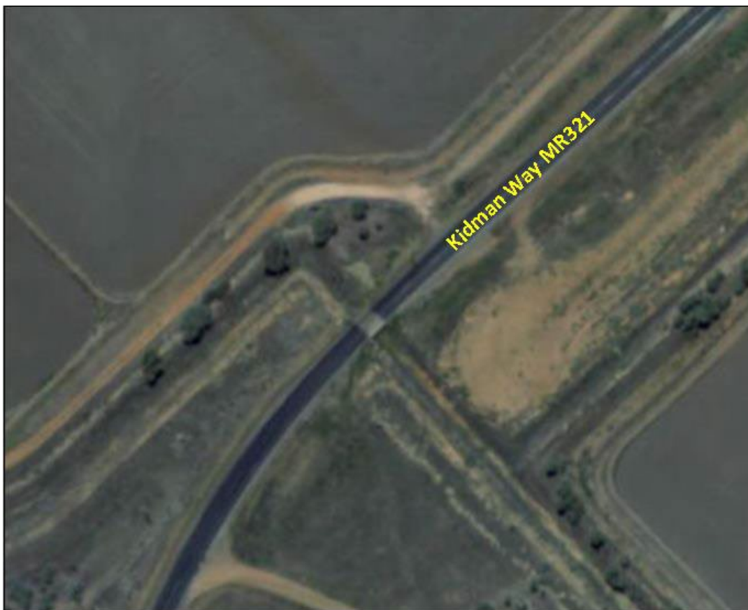
Image (above): Constraint 7.4 Griffith - Railway crossing has sharp approach and departure bends at Widgelli Silos
